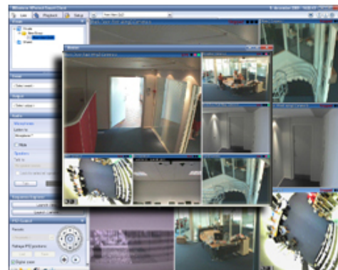
Example of a Smart Client displaying live video from several cameras. Note that a trial version of Milestone XProtect Professional allows viewing of video from a maximum of four cameras.
