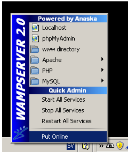
Figure 8. Give WampServer external access.
