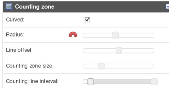
1. The *Line offset* moves the entire counting zone upwards or downwards. How much it can be moved will depend on the counting zone size.
