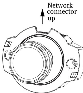
**Note:** To achieve correct image orientation, the AXIS 212 PTZ/AXIS 212 PTZ-V must be mounted with the network connector facing upwards.
