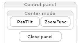
The Control panel can also show your own shortcut buttons, which are configured from **Setup > PTZ Configuration > Advanced**.
