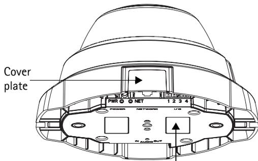
Dome casing for AXIS 212 PTZ-V
