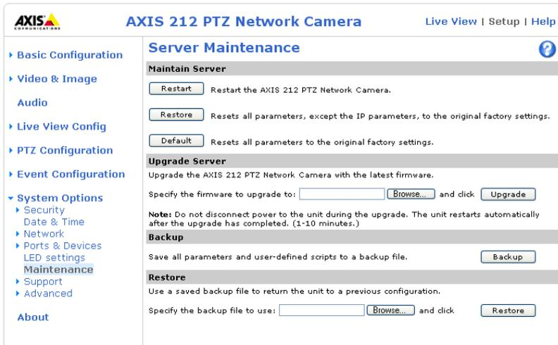
1. Save the firmware file to your computer. The latest version of the firmware is available free of charge from the Axis Web site at [www.axis.com/techsup](http://www.axis.com/techsup)
